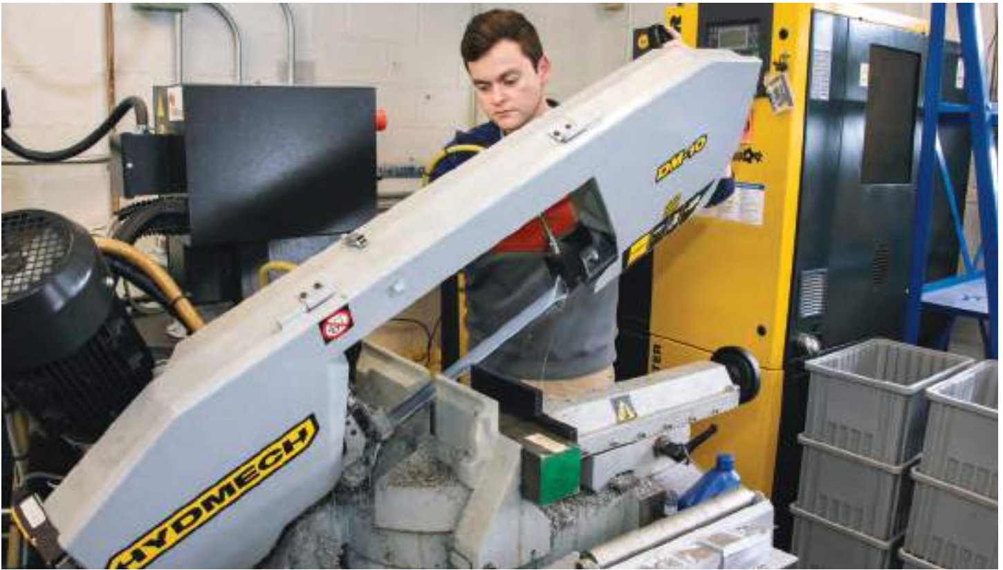
Co-Founder Sean Cerven cutting bar stock to the required dimensions before creating a customer's part.
