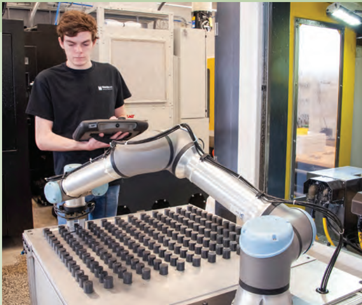
Co-Founder James Cerven setting up Robot, our 'employee' of the month, for its next job. The robot allows Cerven Solutions to run parts continuously day, night and over the weekend.
