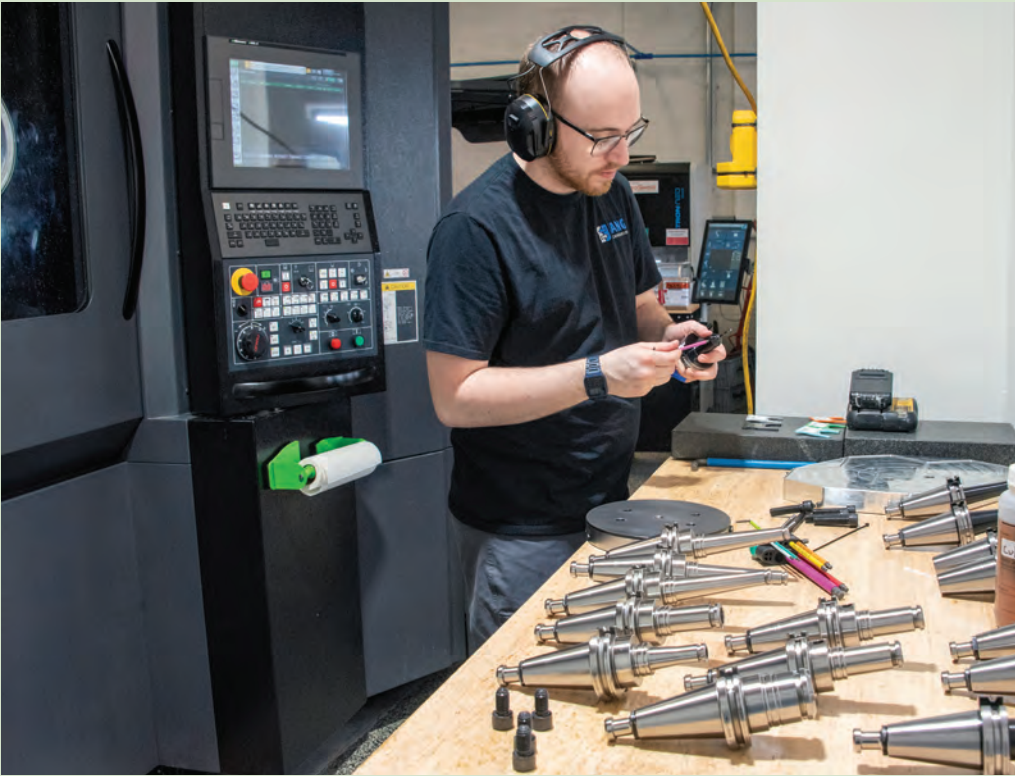
Machinist Jacob Kitchen tooling up the high precision, 5-axis machine for an aerospace job. Earlier he simulated the toolpaths with a CAM (Computer Aided Manufacturing) program to reduce as much as possible the risk of crashing or scrapping parts.
