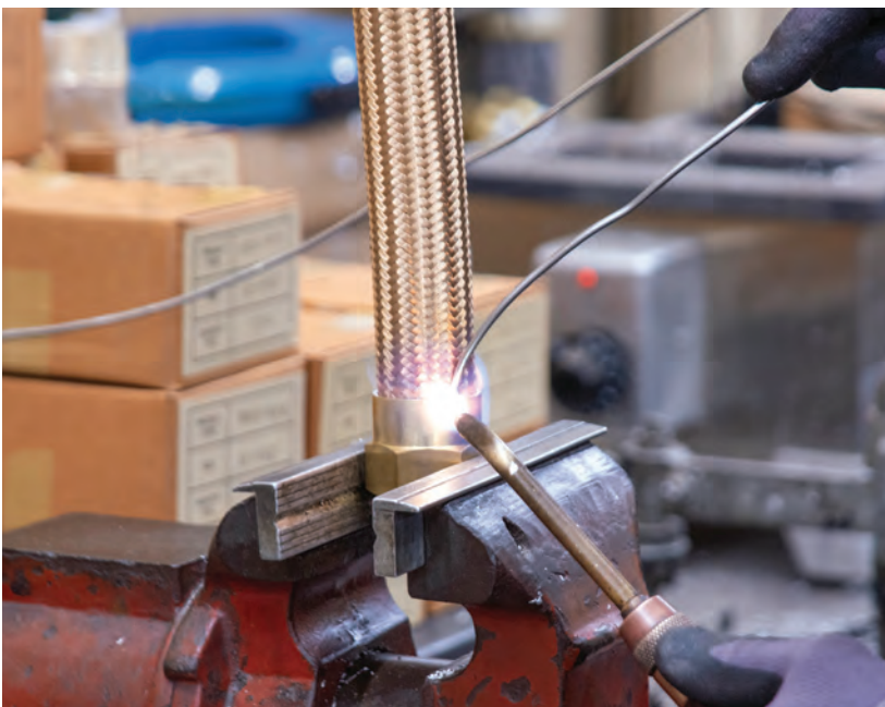
Finishing touches being applied to an Explosion-proof Flexible Coupling for hazardous locations.
