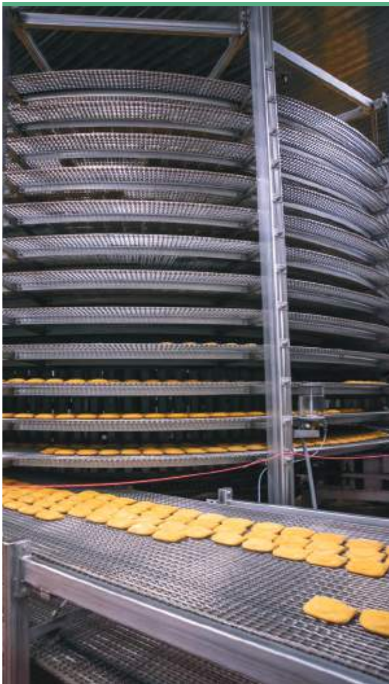
Patties entering the spiral cooler after exiting the oven, move along conveyors on their way to the freezer before being packaged. The company produces both fully cooked (reheatable) and ready-to-bake Jamaican patties, ensuring convenience without compromising authenticity of flavor.
