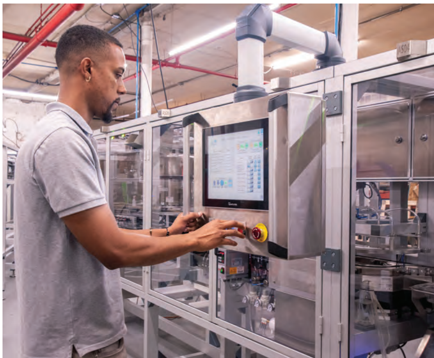
Assembly specialist, Edisaur De La Rosa Sosa works on final testing of a fully automated system for filling, assembly and inspection of single dose nasal spray devices.
