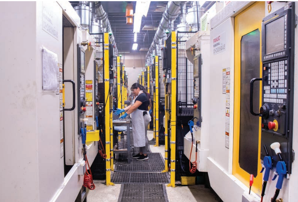
Maria Zhiminaicela is inspecting an automated CNC machining cell. Putnam continues to invest in latest technologies including over 30 robotic cells. These cells are continuously self-adjusting to facilitate tighter CpK’s and providing the ability to run lights out.
