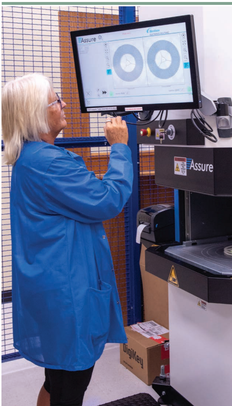
Joan Feeley using our automated component counter x-ray machine. The machine shines x-rays through the packaging and each component creates a black dot on the x-ray photo. The software counts the black dots to tell us how many components remain on the reel.
