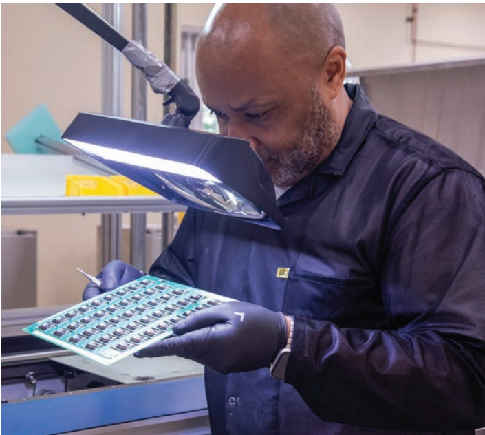
Carlos Pantin inspecting an array of boards which have just exited from the component pick and place machine. This is the last step before the boards go through the soldering process. Errors are easy to fix before soldering and much more difficult once the components are soldered on the board.
