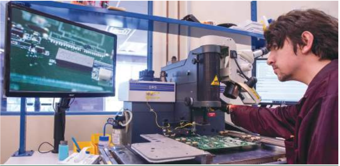
Aaron Zaritsky working at the component rework machine in the process of removing and replacing a component on an assembly. Aaron is viewing a closeup of the component being reworked on the screen to make sure everything looks right.
