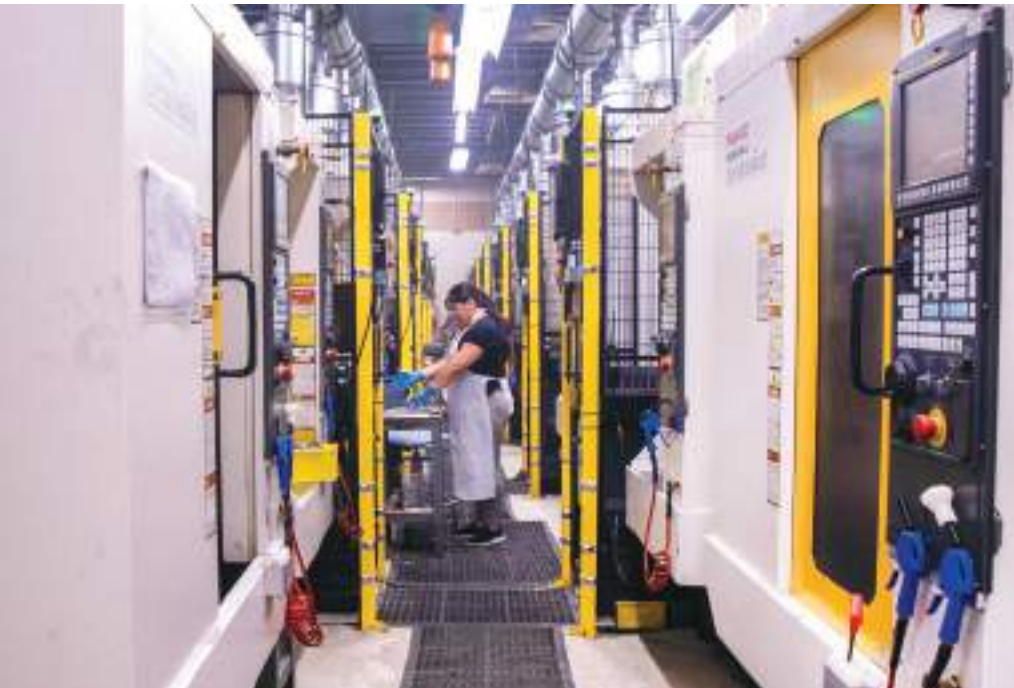
Maria Zhimainicela is inspecting an automated CNC machining cell. Putnam continues to invest in latest technologies including over 30 robotic cells. These cells are continuously self-adjusting to facilitate tighter CpK’s and providing the ability to run lights out.
