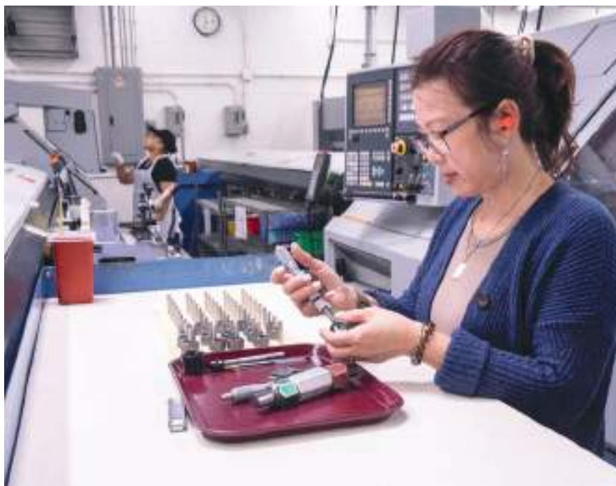
Trang Doan is running an 11 axis Swiss machining center. These machines produce complex components with high degree of precision for the aerospace, medical and commercial industries.
