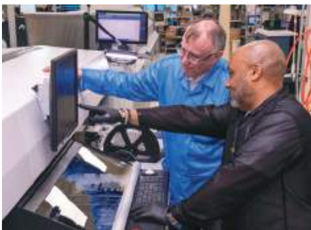
Oliver and Carlos Pantin in front of Metrix's pick and place machine. The machine is capable of picking and placing as many as 35,000 components per hour.
