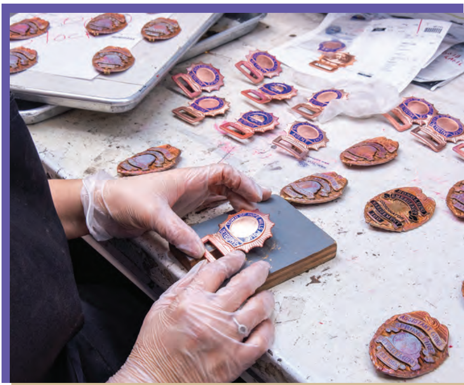
A solderer inspects their work before the next step in production.
