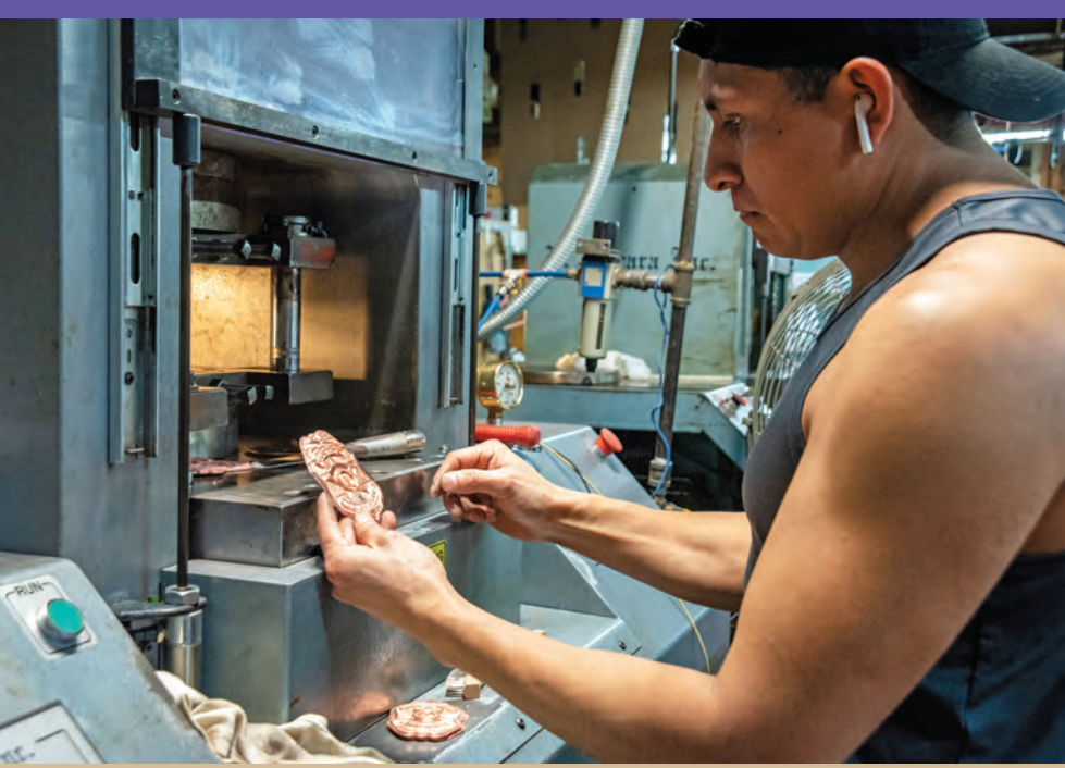
Ensuring all the important badge details emerge after being squeezed by a 650 ton hydraulic press.
