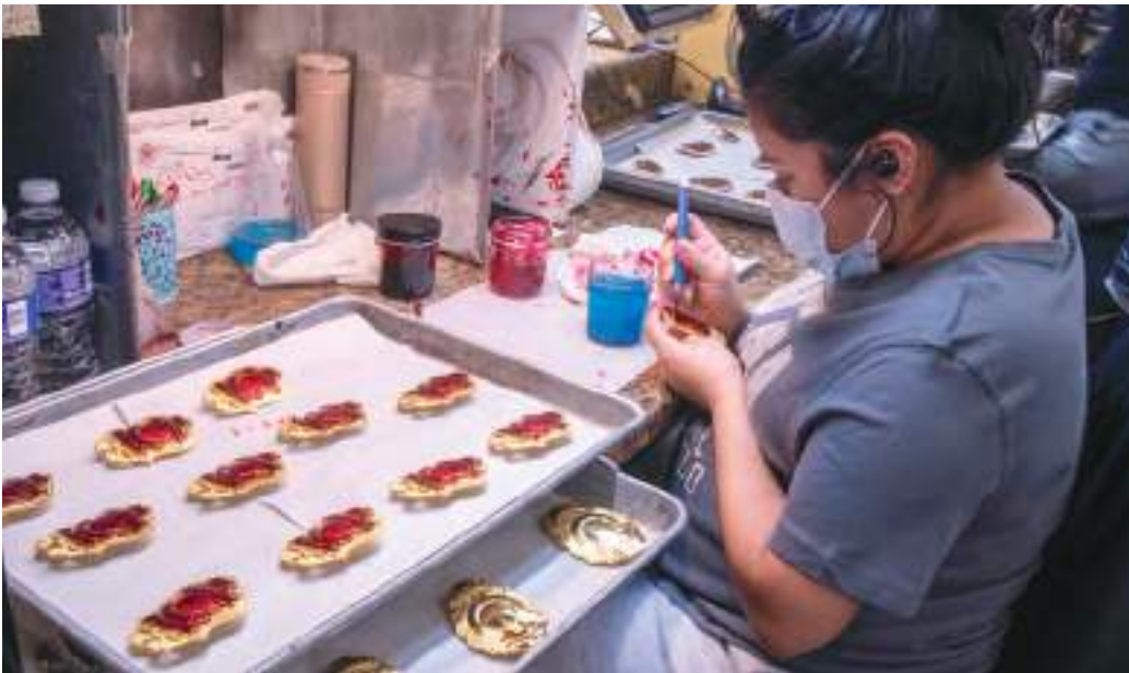
A worker carefully checks badges following the application of an electroplating mask
