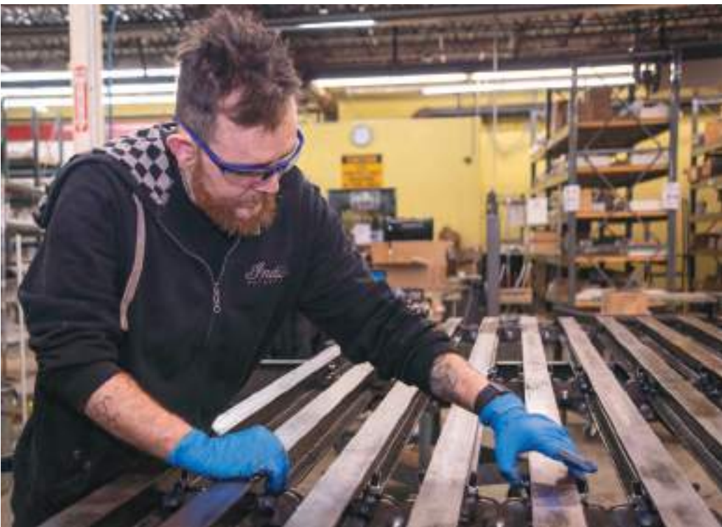
Taylor relies on a skilled group of employees to assemble their machinery. Scott, shown above, is assembling I-Beams for a Clamp Carrier. These I-Beams hold the clamp arms that glue the panels.
