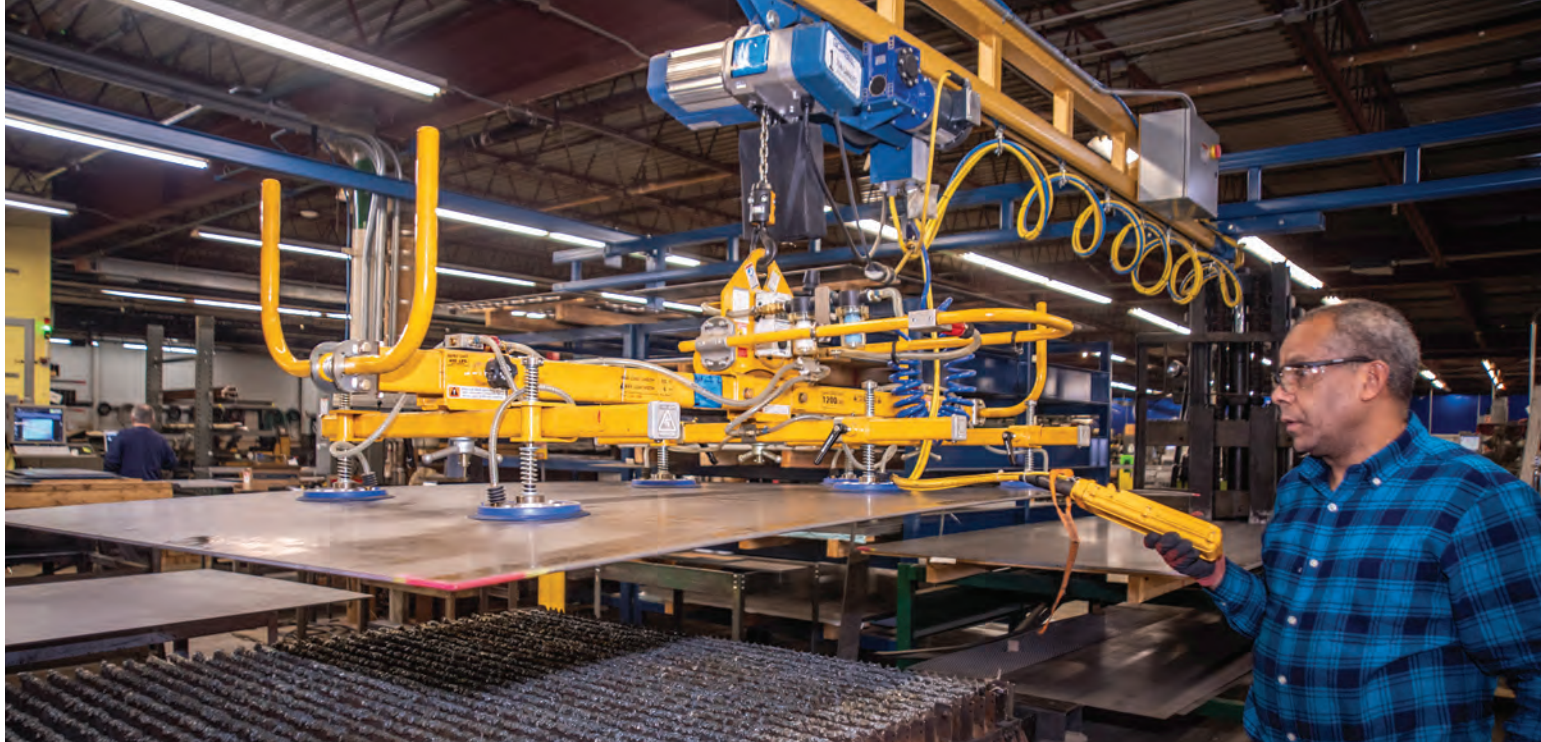
Long time employee Karim uses a vacuum gripper to load sheet metal into a CNC Laser. The CNC Laser is one of the cornerstones of the Taylor factory.
