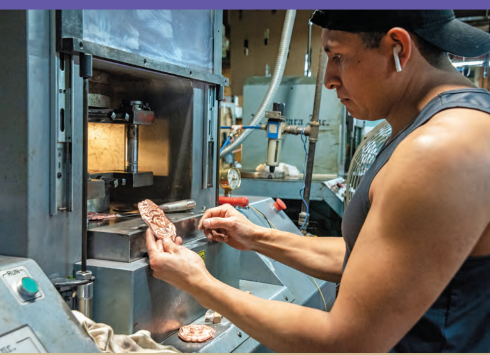
Ensuring all the important badge details emerge after being squeezed by a 650 ton hydraulic press.
