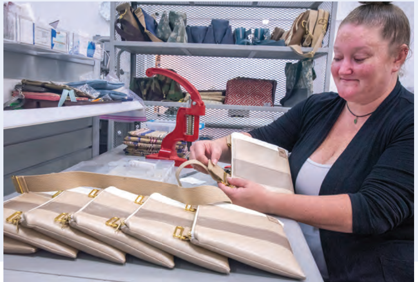
Jillian, Seamstress and Quality Control Manager, performing the 18-point quality control process for finished handbags.
