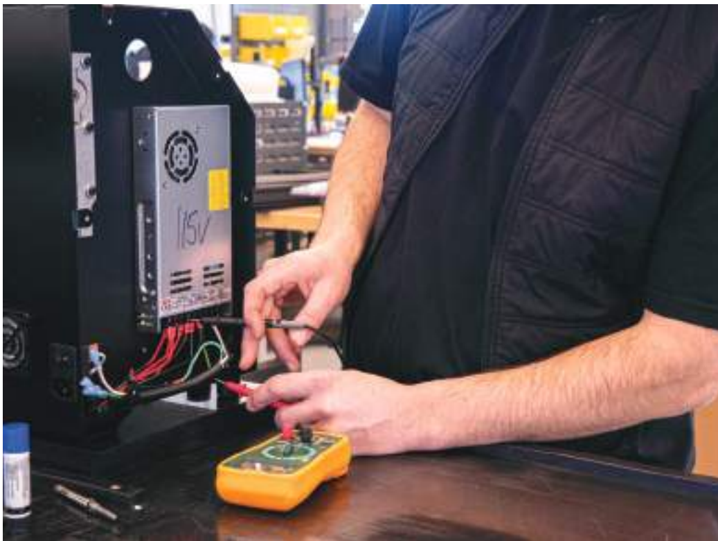
Testing the power supply of the Bantam Tools Explorer CNC Milling Machine.
