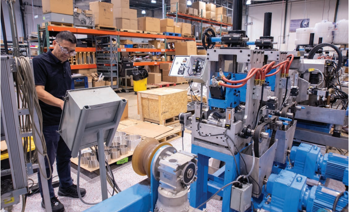
Dr. Stanley Hu, Process Engineer, working on software for an Echomac® ultrasonic phased array system used to detect core and surface defects in steel bar, often used in automotive applications.
