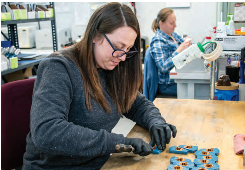
Cathleen Newman, Lysko Assembler, assembling bore gage heads.
