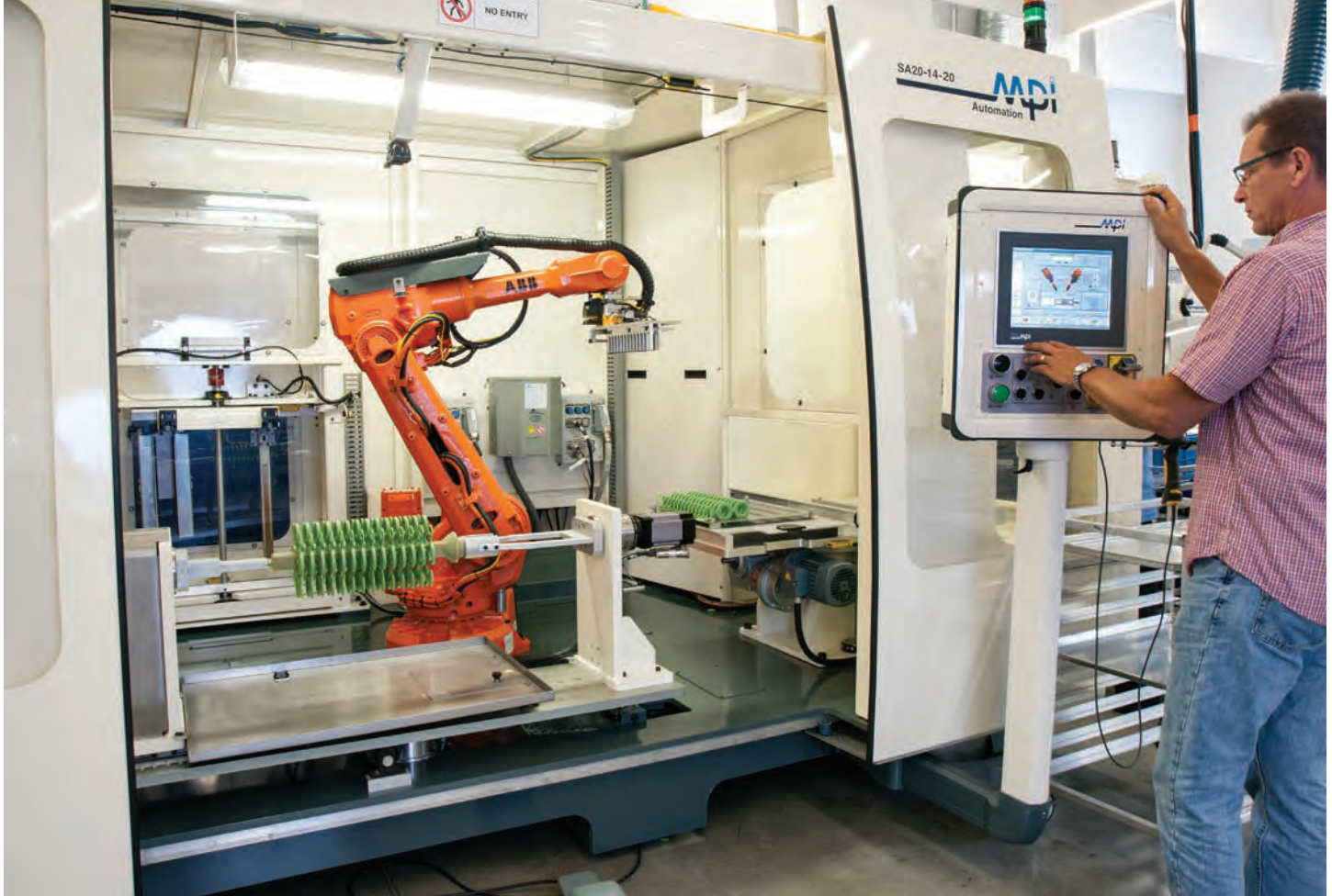
MPI, Inc. machine operator programming the APAS (Automated Pattern Assembly System).
