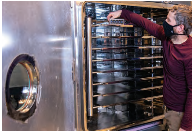
T.J. inspects the shelf stack of a production freeze dryer.
