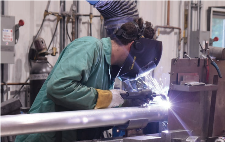
Mitchell Dorn welding poles and columns.
