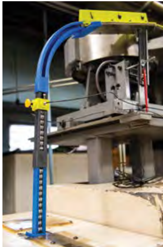
Bearing machine at Schatz Bearing Corp. with a feeder assembly 3D printed out of ABS+ on a Stratasys Dimension 1200ES.
