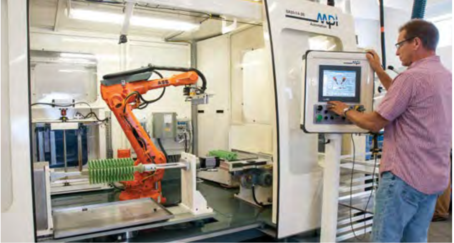
Machine operator programming the APAS (Automated Pattern Assembly System) at MPI, Inc. in Poughkeepsie, NY.
