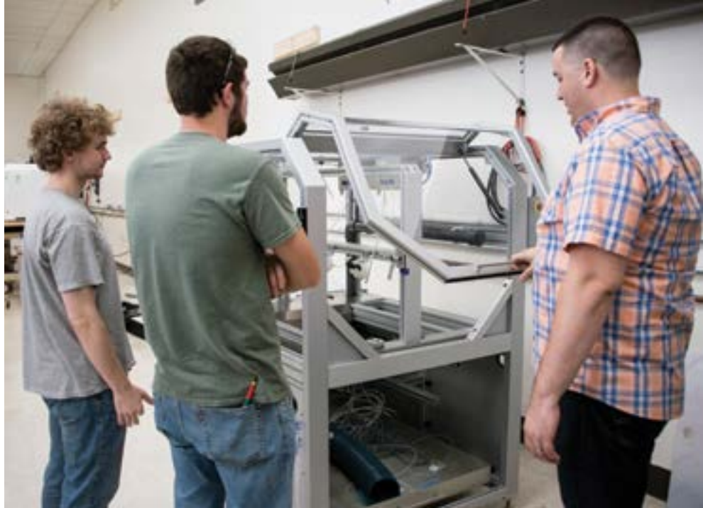
Alex VanPelt, Engineering Intern, Vaughan Clewis, Mechanical Engineer and Adam Carlock checking the alignment, height, and spring tension on the door and the interlock switch. The interlock switch tells the machine the door is closed. During this check they noticed scratches on the lexan and examined to determine whether replacement of the piece was required.
