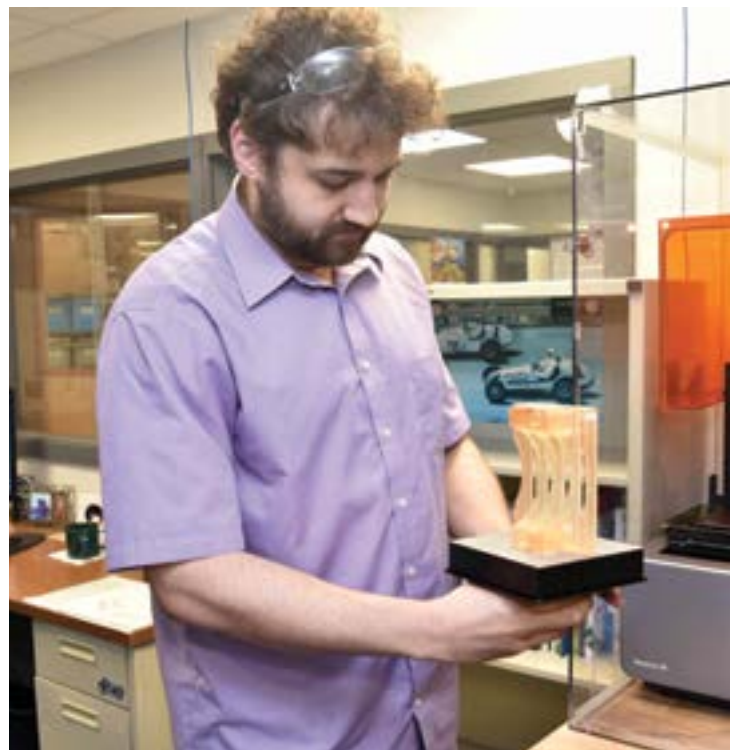
Andrew, one of the Manufacturing Engineers inspecting a production fixture, printed with an in-house 3-D printer.
