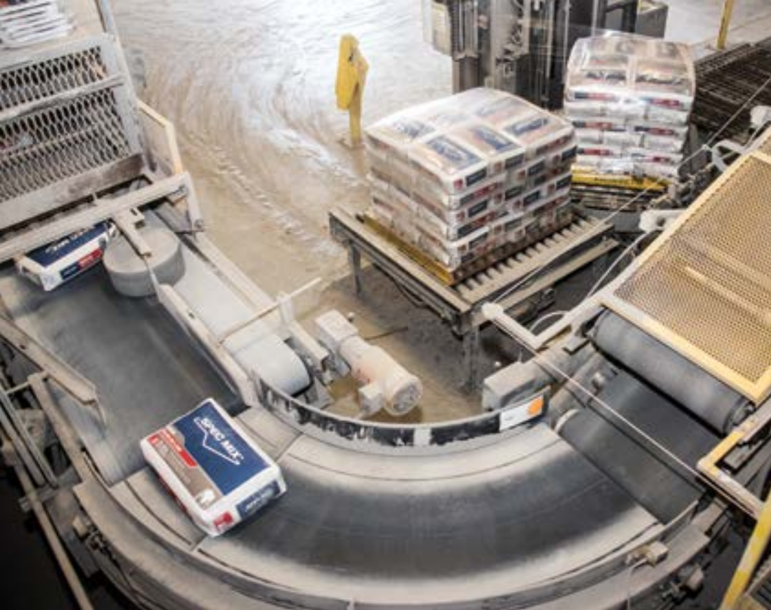
A bag of Spec Mix® travels from the packing area to the automated palletizer to be wrapped and shipped to a customer in Brooklyn.
