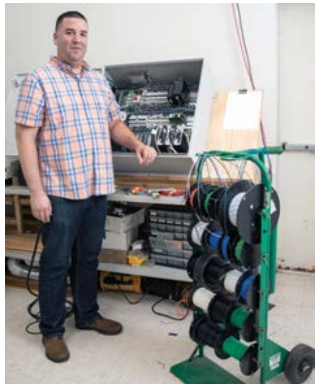
Adam Carlock just completed assembling and wiring the connections for the build station used to make the electronics box and panel. The box holds the electronics for the build and is pressurized to keep the explosive vapors away from any components that could spark. The unit is built to control 3 "slave units".
