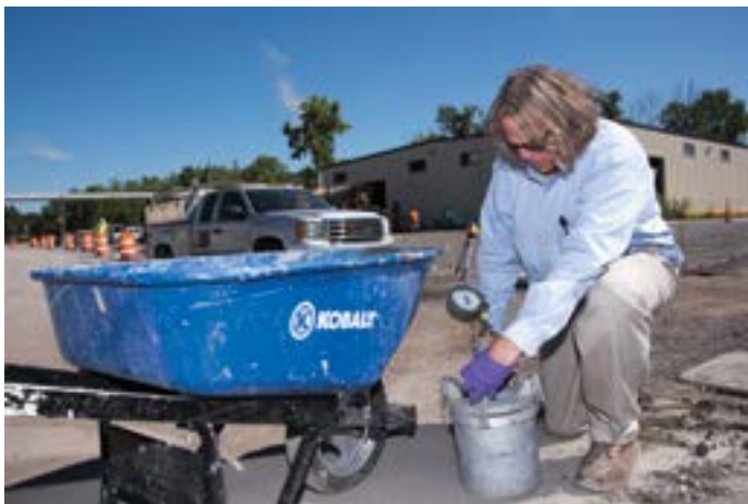
Jerry Guerro, Director of Quality Control prepares a concrete sample for testing on a large concrete pour from an outside contractor.
