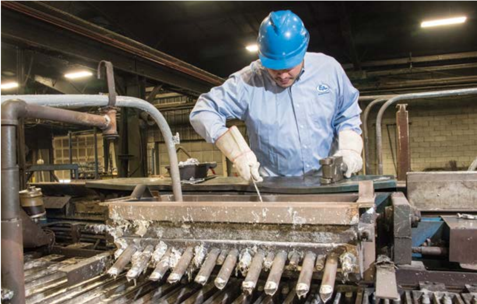
Andre is demonstrating how production samples are taken during the casting process.
