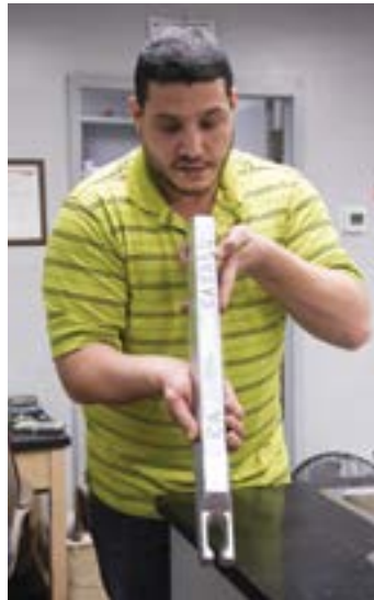
Inspecting a Margash Ingot for imperfections.
