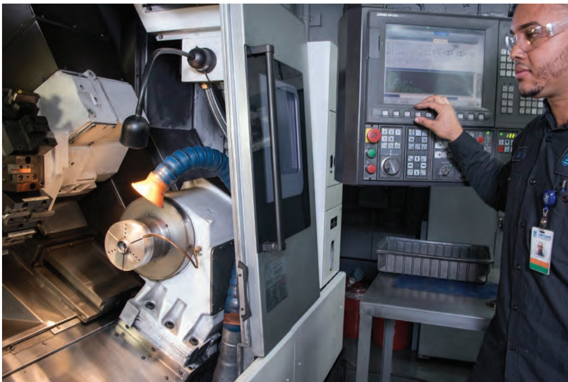
Luis Acosta, CNC Programmer I, machining an aerospace seal face on a dual spindle, 4-axis CNC turning center.
