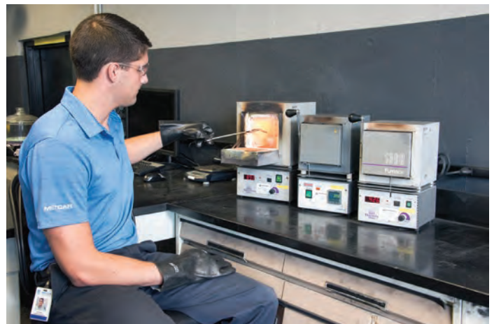
Keith Hoge, Applications Engineer, testing for ash content in the materials lab.
