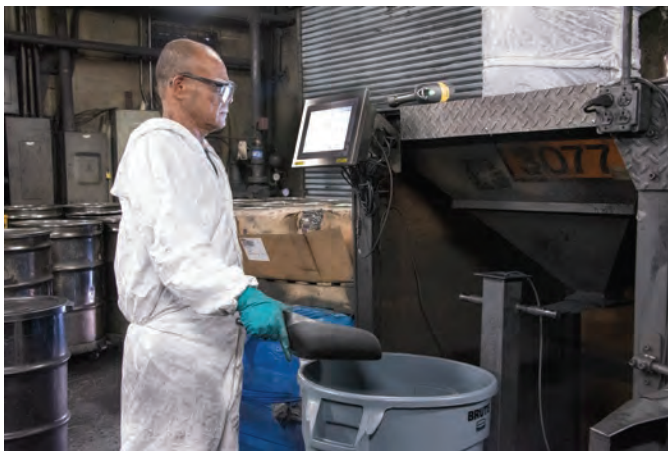
Andres Perdomo, Mixing Operator, weighing raw material formulation on a precision batching scale.
