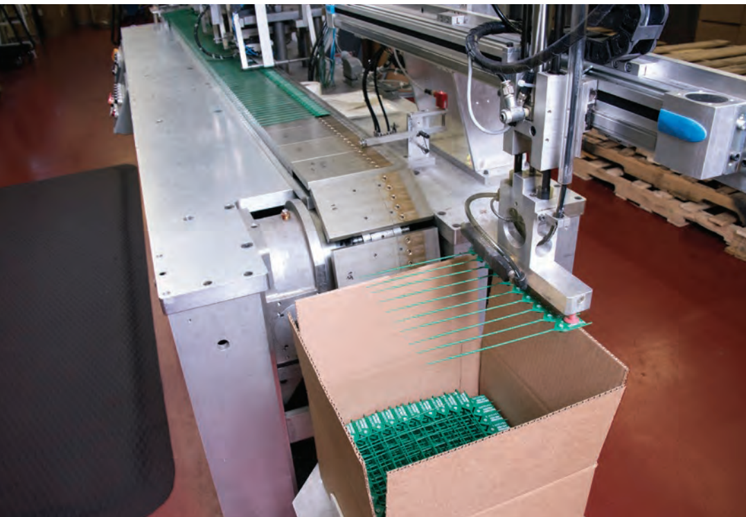
CSS's unique, award-winning packaging was developed specifically to reduce its customers' shipping and inventory costs by consolidating seals within each carton as compactly as possible.
