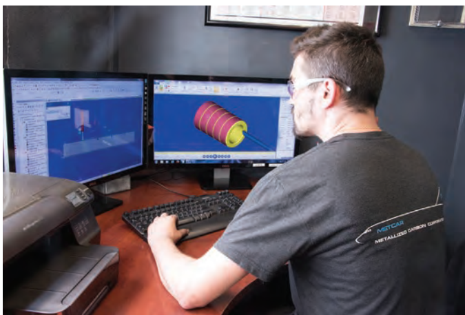
Daniel Oakes, Machinist II, creating a CNC program for a grooved pump bearing.
