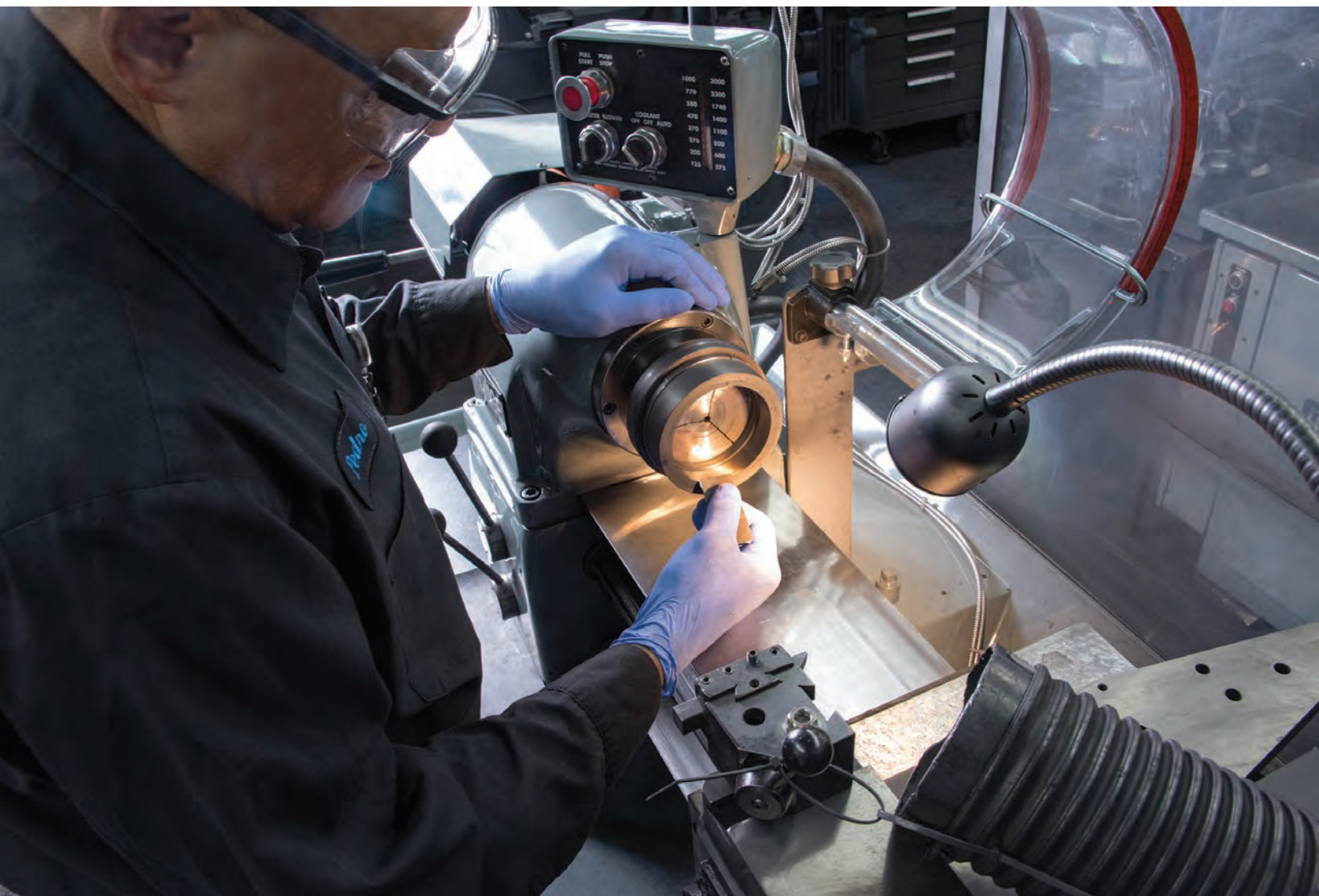
Pedro Ramirez, Lead Machinist, polishing a mechanical face seal on a manual turning center.
