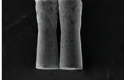
Scanning electron microscopy image of the micromotors. These tiny motors, each about one-fifth the width of a human hair, may someday offer a safer and more efficient way to deliver drugs or diagnose tumors.
