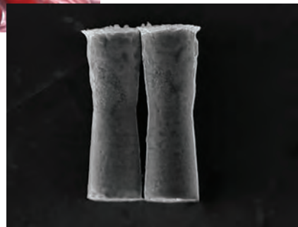
Scanning electron microscopy image of the micromotors. These tiny motors, each about one-fifth the width of a human hair, may someday offer a safer and more efficient way to deliver drugs or diagnose tumors.
