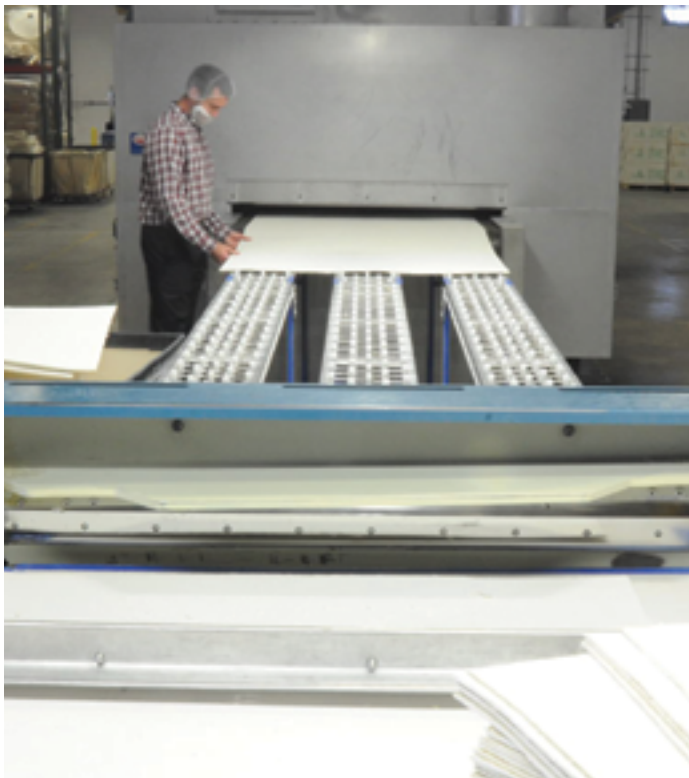
Final filter sheet coming out of the oven for inspection and cutting by operator.
