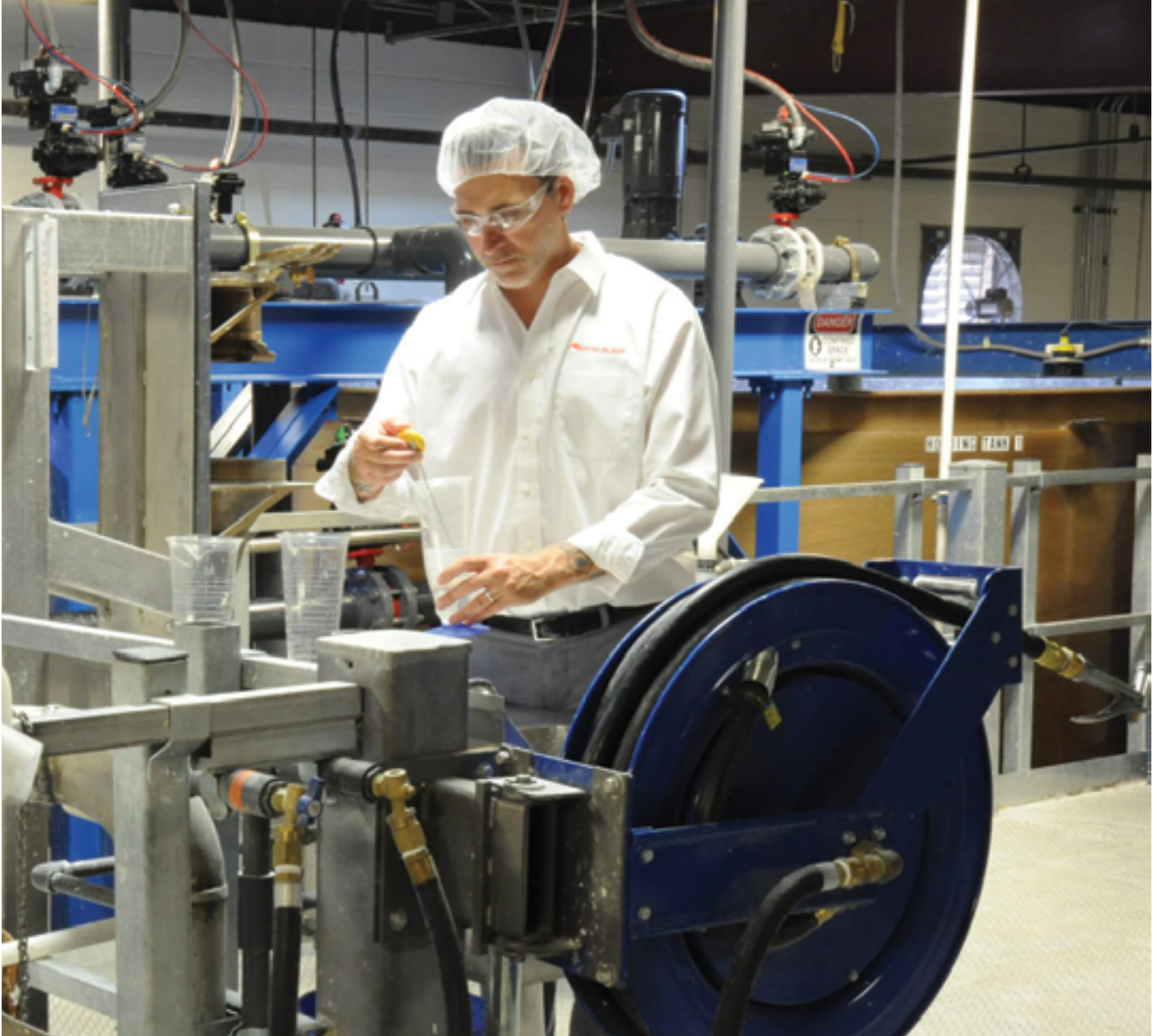
Wet laid process - testing water prior to preparing a batch of filters.
