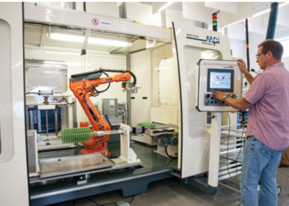
Machine operator programming the APAS (Automated Pattern Assembly System).
