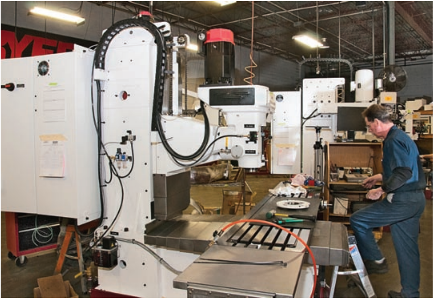
Opposite page: Eric adjusts cutting tool prior to testing; above: Builder Glen Conforti prepares to mount a power drawbar; below: Glen adjusts spindle belt tension on a Fryer MB-16, a toolroom bed mill with manual quill.
