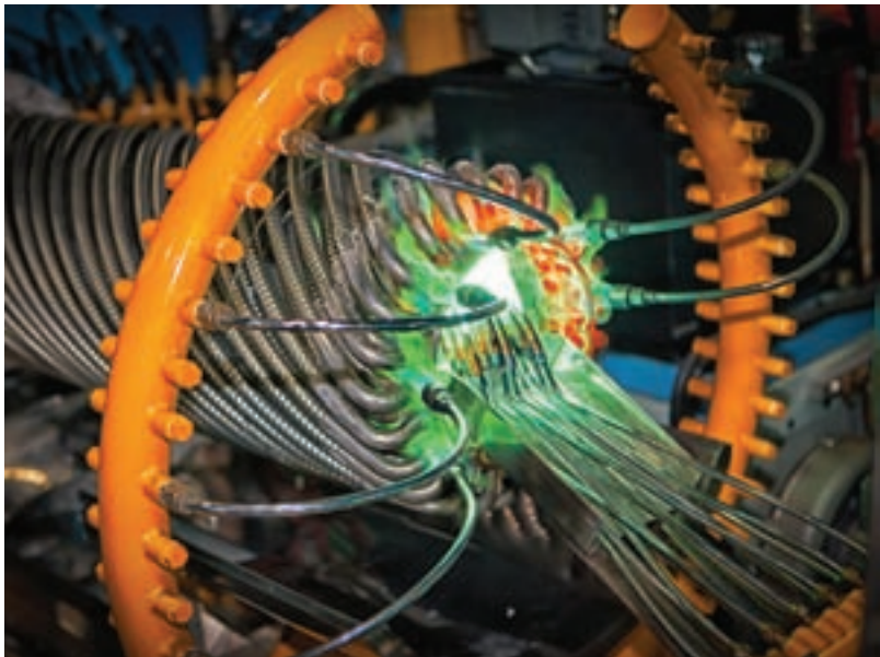
Automated equipment, such as this automated brazing apparatus, helps to streamline the manufacturing process, improve quality and minimize labor.
